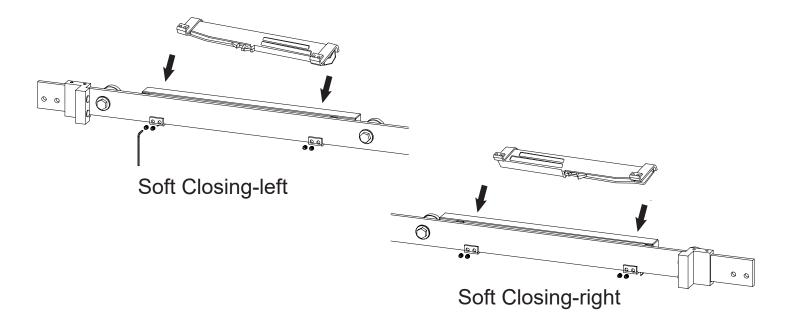
2: Push the door to the left and install the left actuator. Same on the right.
